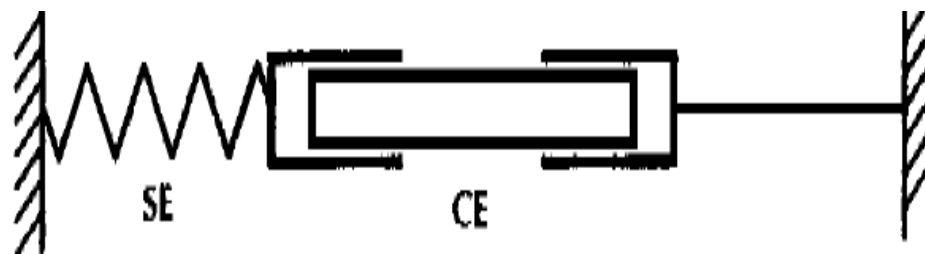
Figure 4-3. Schematic of Hill model with contractile element (CE) with series elastic element (SE). (59)
